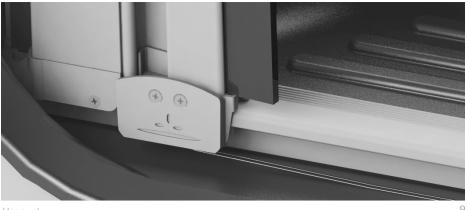
9 Check if the clearance between the pullbar and top profile is within 2-5mm.
