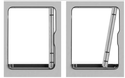
7 When the cassette and pullbar are vertical fasten the cassette to the bottom profile using 2 type 1 screws.
