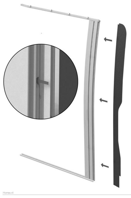
17 Drill two holes (2,5mm) through both the panel and cassette on the top and bottom. Fasten the panel to the cassette with 2 type 1 screws.
