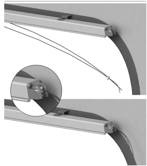
12 Put the cords under tension by unscrewing the cord tensioner, pulling on the cords and fastening the cord tensioner.
